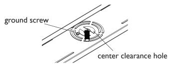
To complete attaching the mounting bracket to the ceiling, mark two additional locations on your ceiling for drywall anchors at points C and D somewhere within the parallel slots. Then if needed, remove one of the machine screws to rotate bracket for anchor installation.
