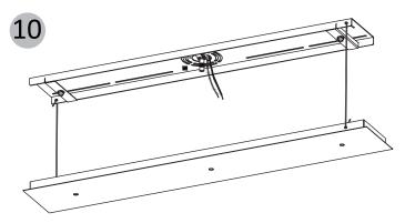
Use the small holes on the vertical flanges of mounting bracket to attach the provided wire hanging hooks. Attach the other ends of the hooks to the small holes on the vertical flanges of the cover plate to suspend the cover plate from the mounting bracket.
