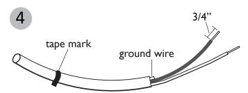
Starting at the cut end, carefully strip back each of the pendant cords' outside insulation to about halfway from the taped marks. If your pendant has a green ground wire, this wire can be cut off entirely as the pendants are not individually conductive. Next, strip back approximately 3/4" of the insulation on each of the remaining two inner wires of each pendant.
