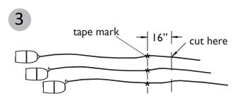
Measure an additional 16" from the tape marks and cut cords at this location. Discard excess wire.
