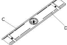
To install the drywall anchors, use a 1/4" drill bit to make pilot holes at points C and D markings. Then screw in anchors until they are flush with the ceiling surface.
