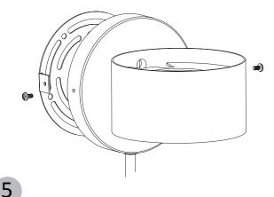
Attach the upper and lower shades the the sconce by inserting the three metal tabs on each shade into the corresponding slots in the sconce. Twist the shades while applying force towards the sconce to lock the metal tabs into the attachment plates.
