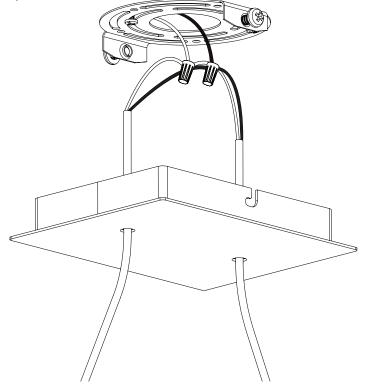
Carefully tuck all wires inside the canopy plate before lifting it up and over the mounting plate. Move the mounting plate laterally to guide the mounting screws along the channel before fully tightening the screws.
