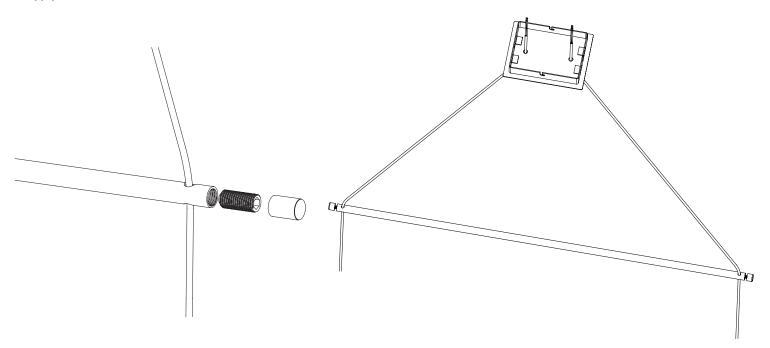
Slide a strain relief down onto each of the pendant cords and use a small flat blade screwdriver to tighten them 1.5" below your tape mark.
