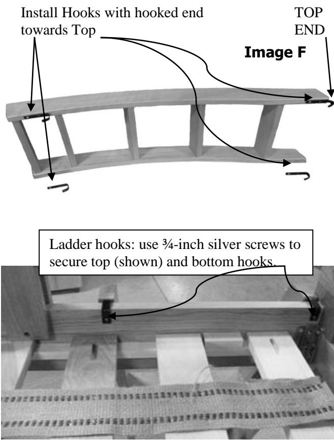
10. Hang the Ladder hooks over the upper and lower Side Rails in the Ladder space reserved adjacent to the shorter Guard Fence. Position the Ladder next to the End and secure the four Ladder hooks to both the upper and lower Side Rails using the 3/4-inch silver screws provided. (See Image G.)
