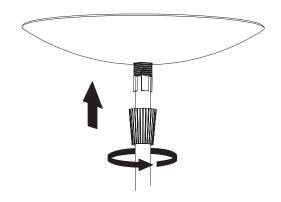
Unscrew the threaded ring from the socket at the lower end of the canopy cord kit. Insert the socket into the metal ring of the inner shade and use the threaded ring to fasten the components together.
