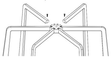
NOTE: The 4 remaining arms of the wooden frame are not removable, do not remove the square-head screws.
