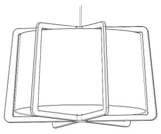
Screw any standard E26 lightbulb into the socket before turning the power back on at the circuit breaker.
