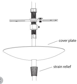
Cut the excess pendant cord approximately 6 inches above the canopy cord kit assembly. Starting at the cut end, carefully strip back about half of the pendant cord's outside insulation. Next, strip back approximately 3/4" of the insulation on the two inner wires.
