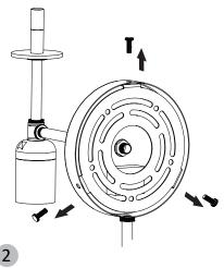
Use pliers to remove the two loose plastic wire nuts on the back of the sconce. This disconnects the included power cord from the fixture, which you will not need when hardwiring this sconce. Remove the black plastic strain relief to pull out the power cord from the bottom of the sconce.
