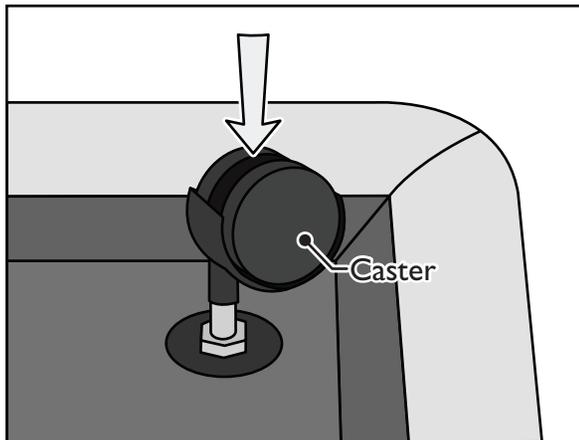
4. Slide the caster onto the caster stem. Using downward pressure, as shown in the image above, push caster onto caster stem until it snaps into place. Repeat with the remaining casters.
