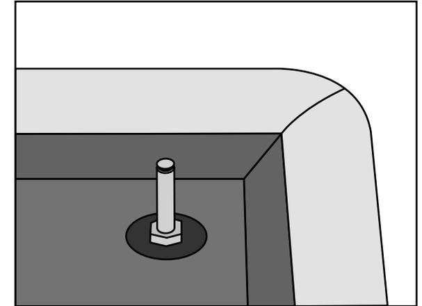
3. Using a 1/2" wrench or 1/2" deep socket, snug down the caster stem. Do this for all caster stems.
