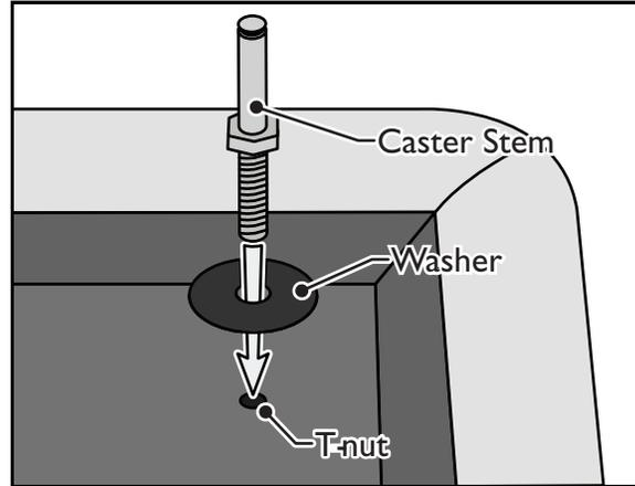
2. Take a caster stem and a washer from the included hardware kit. Insert the caster stem into the washer, and then into one of the remaining T-nuts. There will be four (4) total for square ottomans or five (5) total for round ottomans. Hand tighten the caster stem. Repeat this for the remaining T-nuts.
