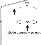
Note: Shade assembly screws may come pre-attached to metal ring around the bulb socket. Remove prior to positioning shade.
