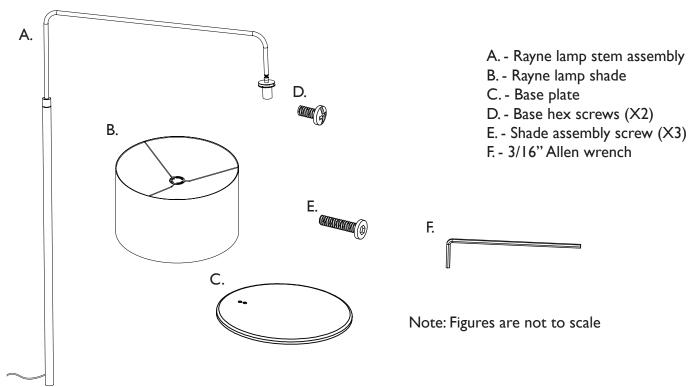
Set the Rayne lamp stem assembly on its side on a carpeted or protected floor to avoid scratches or other damage. Use the 3/16" Allen wrench to fasten the base plate to the stem assembly with the base hex screws.
