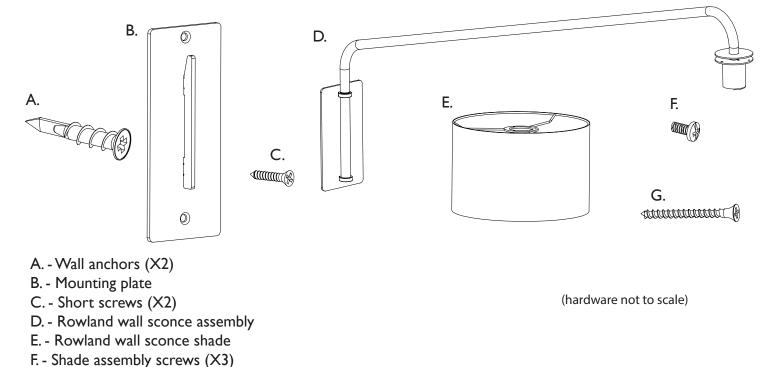
Hold the mounting plate to your wall in the desired location. Use a level to ensure the mounting plate is vertical. Then use a pencil to mark your wall through the two screw holes on the mounting plate.
