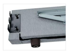
Mount piston mechanisms (two total) to side rails (two total). The long arm extending from the piston mechanism should point towards the footboard, where you installed the six bolts in step 1. Each piston mechanism requires four bolts to properly install.
