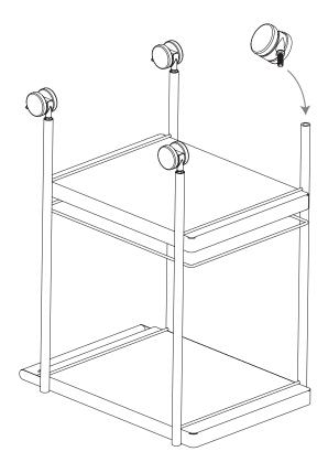
Hand-tighten all casters with the included wrench, taking care not to over-tighten.
