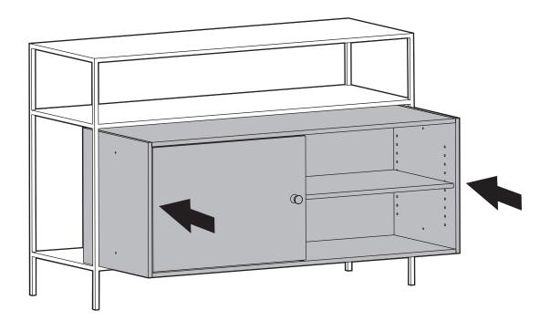
Once the insert is fully inserted into its space, attach the side panels using the included screws and allen wrench. The side panels keep the insert in place.
