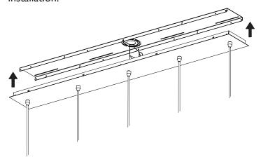
Assess the position of your pendants. If you are not satisfied with the arrangement, determine how much you would like them to move up or down and adjust locking collars or knots accordingly. Unscrew cover plate, rehang it with the wires hooks and reposition the cord locking collars or knots.
