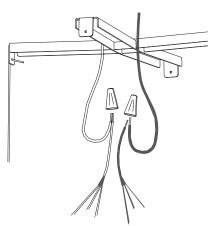
Twist like-color wires from the electrical box to the lead wires on each of the provided wire harnesses. Twist on yellow wire nuts to hold the wires together.
