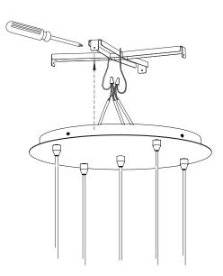
Remove the wire hanging hooks while lifting the cover plate up and around the four tabs on the cross-bracket. Make sure all wires are tucked safely inside. Align the slotted holes on the upper ring of the ceiling plate with the holes in the cross-bracket. Use the four assembly screws to join the two components together. Do not over tighten.
