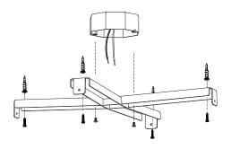
Note: Long wood screws are provided for mounting the cross-bracket to surfaces that don't require anchors.
