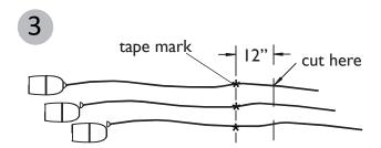
Measure an additional 12" from the tape marks and cut cords at this location. Discard excess wire.
