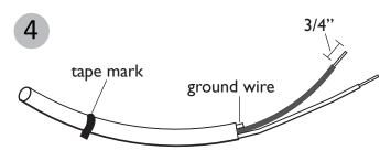
Starting at the cut end, carefully strip back each of the pendant cords' outside insulation to about halfway from the taped marks. If your pendant has a green ground wire, this wire can be cut off entirely as the pendants are not individually conductive. Next, strip back approximately 3/4" of the insulation on each of the remaining two inner wires of each pendant.
