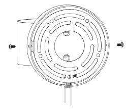
Choose where to mount your sconce, ensuring the power cord will reach the outlet you intend to use. Hold the wall mounting plate against the wall and use a level to ensure the plate is vertically aligned. Mark the location of the two screw holes with a pencil.
