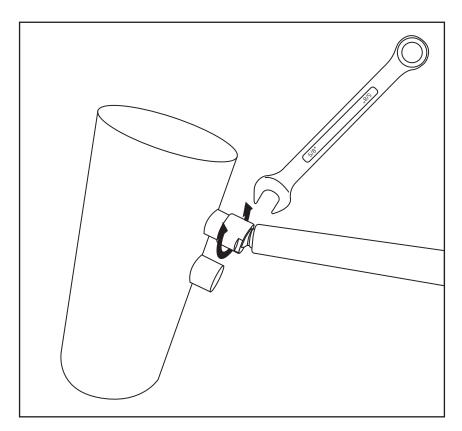
The lamp head can loosen over time. Use a 5/8" wrench to adjust the tension of the lamp head if necessary. Consider placing a fabric cloth or other protective barrier between your lamp and the wrench to protect its finish.
