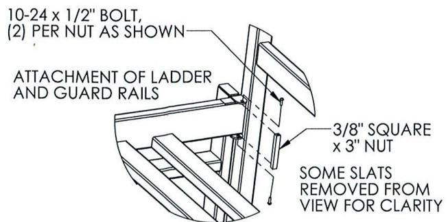
9. Remove the screws from the screw/nut assembly of the ladder. Position the ladder on the right or left side depending on your preference. Attach the ladder by first placing the lower clips over the bottom rail, then put the C brackets over the 3" top rail. Making sure ladder is against the end, put the long square nut in between the holes of both C
