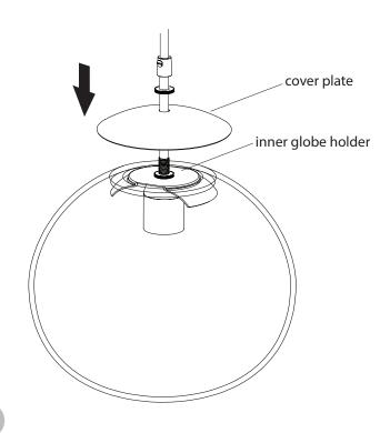
Slide the cover plate down onto the glass globe, and then tighten the thumb nut, strain relief and set screw. Complete each pendant assembly entirely before moving on to the next pendant assembly.
