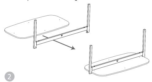
Place leg 2 into the bottom cut-out of leg I and center the top.
