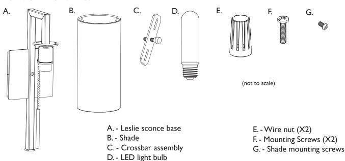
**NOTE:** This sconce is designed for hardwire mounting to an existing wall sconce junction box. If you do not have an existing junction box have one installed by a licensed professional.
