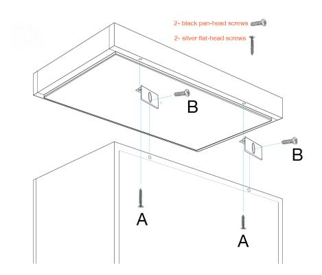
2) Use the silver flat-head screws (A) to fasten each metal bracket to the bottom of the changing tray using the pilot holes provided. Use the black pan-head screws (B) to secure the changing tray to the back of the dresser through the slot in the bracket and into the back of the dresser.
