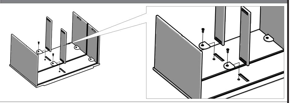
Fit short edge of Rib into Side's center pocket cut outs with cut out facing same side as the Side's threaded hole. Place Blocks G into the Ribs pocket cut outs, insert bolts through the blocks into the Side's threaded holes, and finger tighten.
