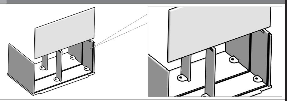
Slide Floor into End's groove track cut outs and into the Side's groove track cut out (Floor can be placed in middle track to save dirt). Attach second Side using steps 1 & 2.
