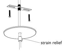
Using the included wire nuts, twist together the wires from the pendant with their corresponding wires from the junction box. Tuck the excess wire up into the junction box before lifting the canopy plate up to the ceiling and tighten in place with the strain relief.
