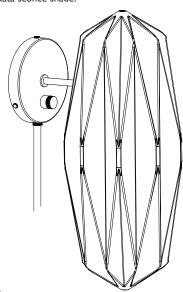
Locate the opening of the Orikata sconce shade and spread the shade open and around the arm of the sconce body assembly. The brass cylinders above the wooden disc on the sconce body assembly should extend upward toward the top opening of the shade, and the horizontal arm of the sconce body should extend out of the shade through the circular hole at the back.
