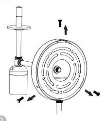
Choose where to mount your sconce, ensuring the power cord will reach the outlet you intend to use. Hold the wall mounting plate against the wall, and use a level to ensure one of the protruding tabs is horizontal and at the top of the mounting plate. Mark the location of any two screw holes with a pencil.
