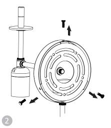
Use pliers to remove the two loose plastic wire nuts on the back of the sconce. This disconnects the included power cord from the fixture, which you will not need when hardwiring this sconce. Remove the black plastic strain relief to pull out the power cord from the bottom of the sconce.
