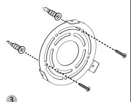
Remove the wall-mounting plate from its intended location. If you are mounting to drywall, use a power drill with a 1/16" drill bit to create pilot holes at the two screw marks. Screw the wall anchors into the holes until they are flush with the surface of the wall. Align the wall-mounting plate to the anchors and attach the mounting screws through the plate and into the anchors. If you are mounting to a surface other than drywall, alternative hardware may be required.
