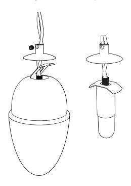
Unscrew glass diffuser and remove G9 bulb from ceramic socket by gently pulling on plastic shell.
