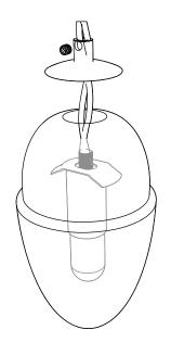
Turn metal hanger vertical until it fits through the opening in the glass. Slide glass off the fixture assembly and store someplace safe.
