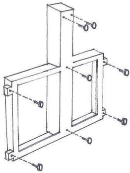
**1** Screw the plastic feet (S) to the underside of the base frame (P).
