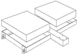
**3** Place the base weights (O) in the base frame (P). **The cutout handles must go from front to back.**
