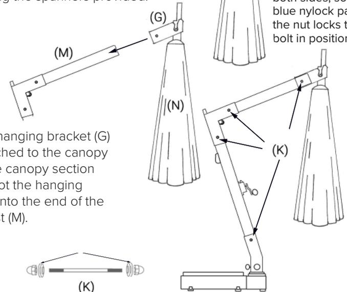
**8** With the hanging bracket (G) now attached to the canopy (N), lift the canopy section up and slot the hanging bracket onto the end of the cross post (M).
