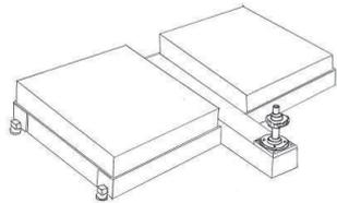
**4** Fix rotation mechanism (A) to the base using the M8 bolts and washers (C) and place the rotation cover over the top (Q).
