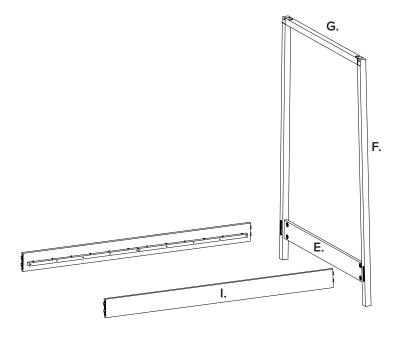
Connect the side rails to the headboard assembly by inserting the male end of a side rail bracket into the female end of a leg bracket. Push downwards to lock into place.
