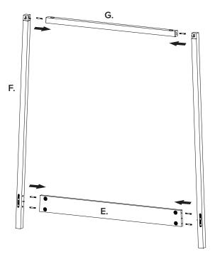
Attach the side rails to the footboard assembly by inserting the male end of a side rail bracket into the female end of a leg bracket. Push downwards to lock into place.
