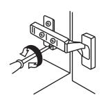
3. Depth adjustment: On clip-style hardware, loosen rear screw, adjust and retighten.
