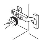
2. Height adjustment: Rotate cam screw on mounting plate to adjust door position (±2mm).
