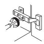
2. Height adjustment: Rotate cam screw on mounting plate to adjust door position ( $\pm 2$ mm).
