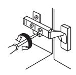
**3. Depth adjustment:** Turn rear spiral-tech cam screw to adjust door position (+3mm, --2mm).
