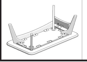
Place Block G into Short Support. Insert Short Support and Block into Table Top grooved track. Insert Bolt through Block into Table Table and finger tighten. Repeat step for second Short Support.
