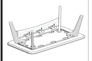
Place Blocks G into Long Support. Insert Long Support and Blocks G into Table Top grooved track. Insert Bolts through Blocks into Table Table and finger tighten. Repeat step for second Long Support.
