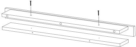
Place the wooden wall mount strip on the wall at the ledge's intended location. Use a level to ensure the wall mount strip is properly positioned. Use a pencil to make a mark on the wall along the two vertical edges of the wall mount strip, then use a tape measure to measure the distance of the screw holes from the edge of the wall mount strip. Make a mark on the wall at that distance in from each edge mark. These marks will be the mounting screw locations.
