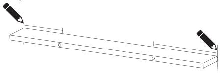
Use a power drill and a 3/16" drill bit to drill pilot holes at your mounting screw location marks. If you've planned your mounting screw locations to correspond with wall studs, there is no need to use the included wall anchors. Otherwise, use a #2 Phillips screwdriver to screw in the wall anchors until they are flush with the surface of the wall.
