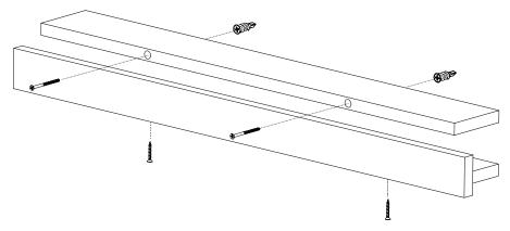
Hold the ledge assembly against the underside of the wall mount strip and use the previously removed assembly screws to reattach the ledge to the wall mount strip.
