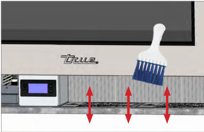
FIG. 2. Never brush across the coil fins.
