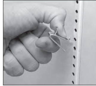
FIG. 1. Installing top tab of shelf clip.
