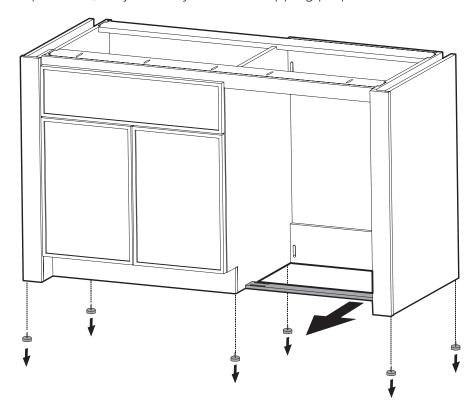
Insert refrigerator. With the unit near its final position but far enough away from the wall to access the cabinet's back, slide the refrigerator into place. The leveling feet on the bottom of the refrigerator can be used to tune the fit and stability.
