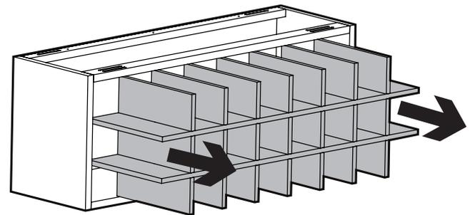
To remove the wine storage partition, simply pull from the front. The partitions are comprised of multiple individual parts, but must be pulled out as a complete assembly.
