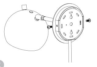
Choose where to mount your sconce, ensuring the power cord will reach the outlet you intend to use. Hold the wall mounting plate against the wall and use a level to ensure the plate is vertically aligned. Mark the location of the two screw holes with a pencil.
