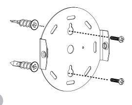
Remove the wall mounting plate from its intended location. If you are mounting to drywall, use a power drill with a 1/16" drill bit to create pilot holes at the two screw marks. Screw the wall anchors into the holes until they are flush with the surface of the wall. Align the wall mounting plate to the anchors and attach the mounting screws through the plate and into the anchors. If you are mounting to a surface other than drywall, alternative hardware (not provided) may be required.
