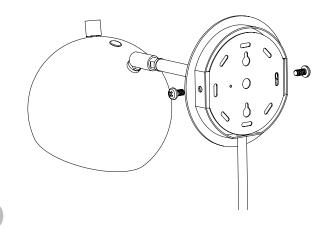
Use pliers to remove the plastic wire nuts on the back of the sconce. This disconnects the included power cord from the fixture, which you will not need when hardwiring this sconce. Pull out the power cord from the bottom of the sconce. Use the included cord hole plug to cover the cord exit. 3
