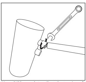
Use a 5/8" wrench to adjust the tension of the lamp head if necessary. Consider placing a fabric cloth between your lamp and the wrench to protect its finish.
