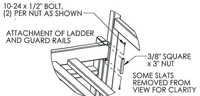
end, put the long square nut in between the holes of both C brackets, insert the screws through the C bracket holes (top and bottom) and screw them into the long square nut. Tighten screws with screwdriver.
