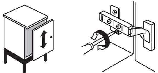
**3. Depth adjustment:** Turn rear spiral-tech cam screw to adjust door position (+3mm, -2mm).
