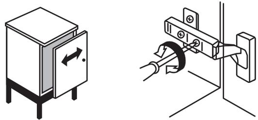
**2. Height adjustment:** Rotate cam screw on mounting plate to adjust door position ( $\pm 2\text{mm}$ ).
