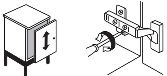
**3. Depth adjustment:** On clip-style hardware, loosen rear screw, adjust and retighten.
